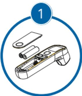
Unpack thermometer and insert batteries.
