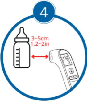
Point the thermometer 3-5cm away from the object and press ⏹.
